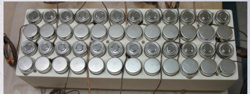
12p-4s battery brick with epoxy syntactic foam interstitial material
