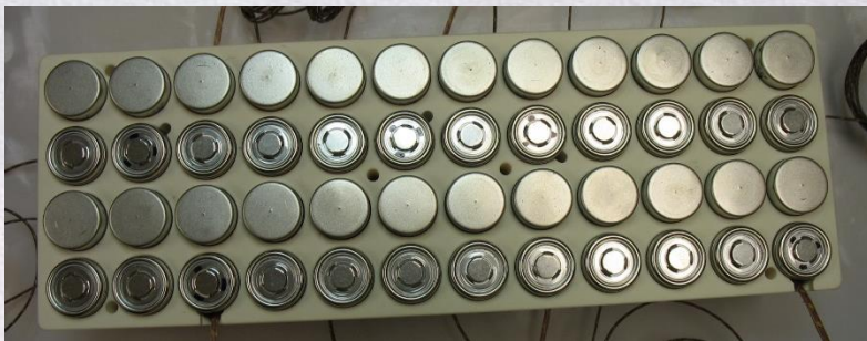
12p-4s battery brick with epoxy syntactic foam interstitial material
