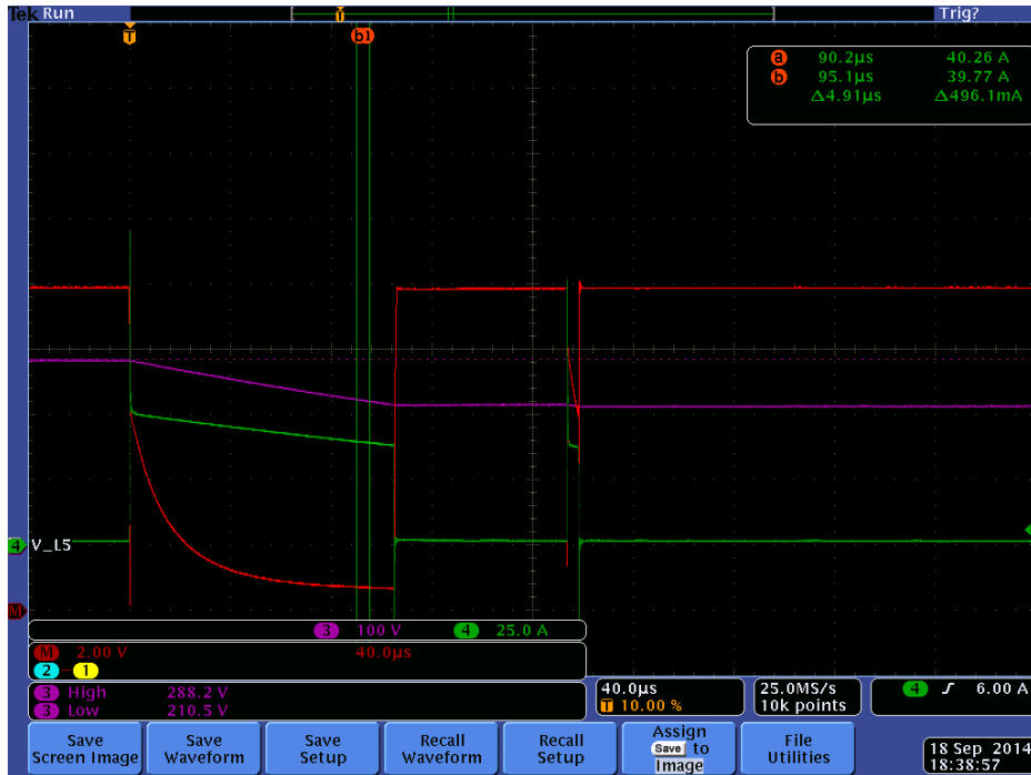
Figure 73.—Oscilloscope Traces for Resistive Test at 40 A
