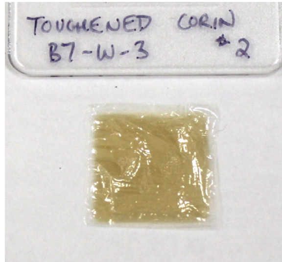
Figure 23. Toughened CORIN® XLS flown on MISSE-7B wake side.
