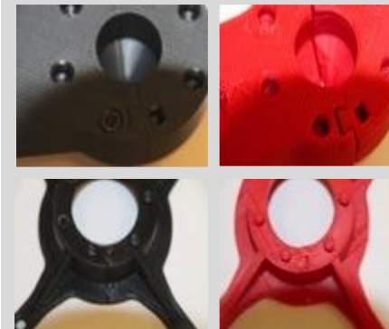
EVA Suit Fan Shipping Container: Design Clearances had to be relaxed for part to be printed on one FDM printer (red) vs. another in order for the parts to be assembled.
