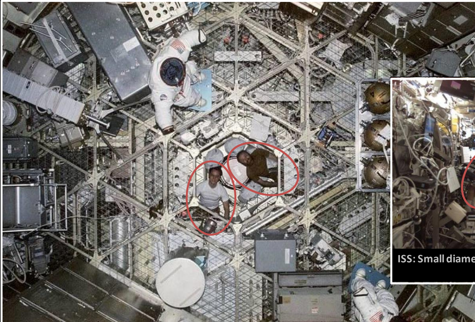
Skylab: Large diameter, vertically oriented layout.
