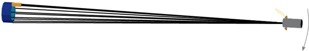
Figure 11. Concept for spin-up of the e-sail structure with a single sub-satellite.
