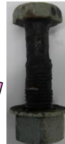
Conceptual illustration of corrosion indication in structural bolts at the launch pad
