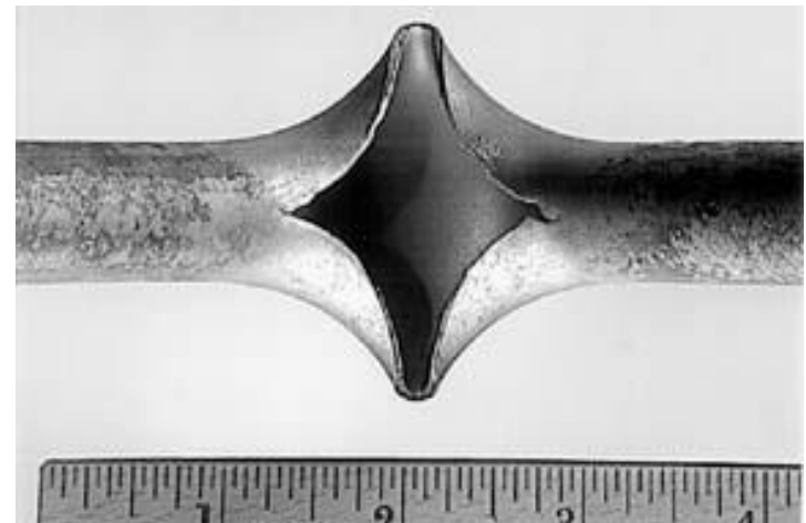
SS 304 tubing split caused by pitting
