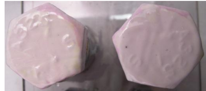
Nut and bolt set up for crevice corrosion testing. The pictures show results after 600 hour of salt fog exposure 76
