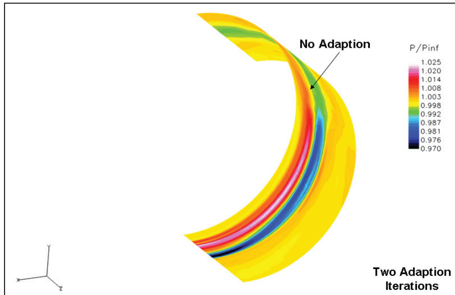
Figure 2-17. CFD predicted \Delta P/P_o cylinder data at three body lengths, Boom7, M = 1.2 .
