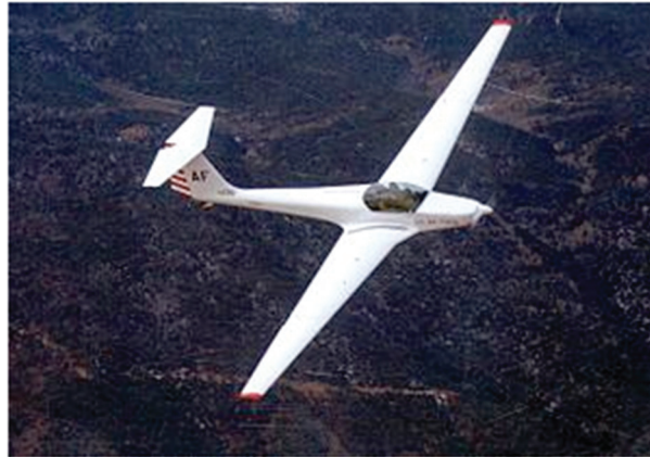
Figure 3-3. TG-14 powered glider used for recording sonic booms in the air. (Source: NASA)
