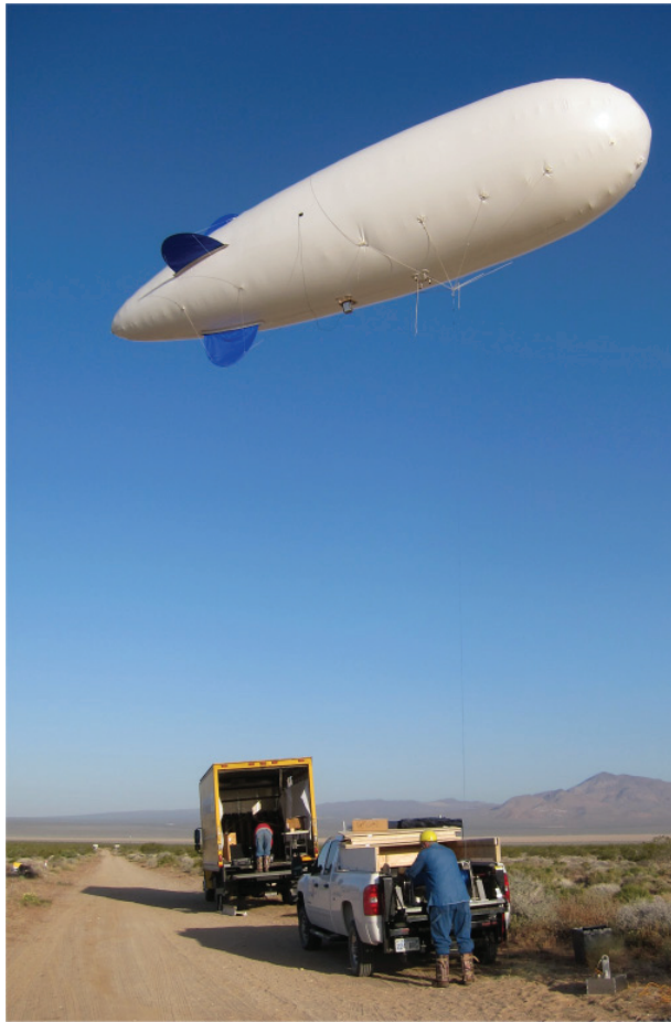
Figure 3-6. Cessna operated tethered blimp for elevated microphones.
