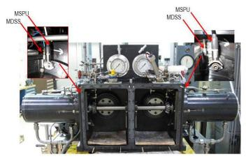
Figure 4.—Locations of accelerometers.
