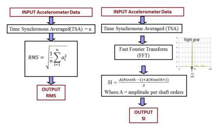
Figure 6.—RMS and SI calculations.
