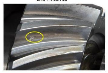
Figure 16.—Damage to one pinion tooth.
