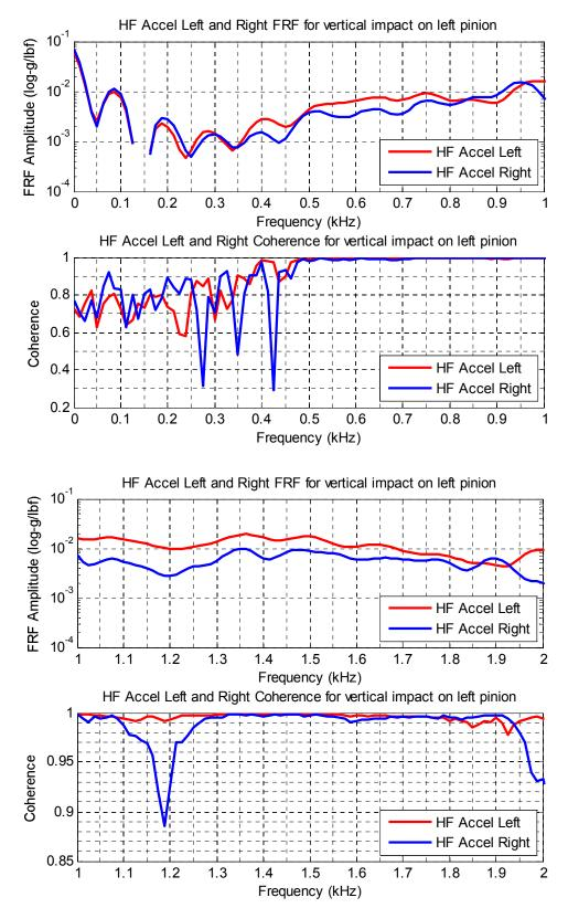
Figure 19.—FRF, Coherence and CDF at 29 percent load measured on right and left.
