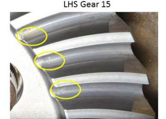
Figure 14.—Gear teeth anomaly on the second gear set.
