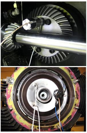
Figure 21.—Actuators installed on the test rig and NGB fixture.
