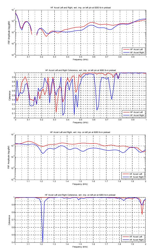
Figure 18.—FRF, Coherence and CDF at 104 percent load measured on right and left.
