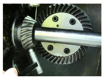
Figure 7.—Impact on left pinion in the vertical direction.
