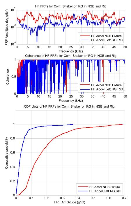
Figure 22.—FRFs, Coherence and CDF of test rig and NGB fixture.
