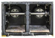
Figure 2.—Three spiral bevel geared systems.
