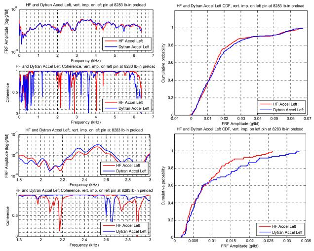
Figure 11.—FRF, Coherence and CDF at 104 percent load measured with HF and Dytran accels.
