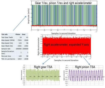
Figure 5.—Information used to calculate TSA.
