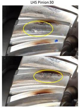
Figure 12.—Damage to gear and pinion teeth.
