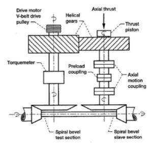
Figure 3.—Cross-section of the test rig.
