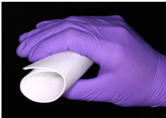
Figure 12.—Aerogel composite reinforced with APA-2 alumina paper.
