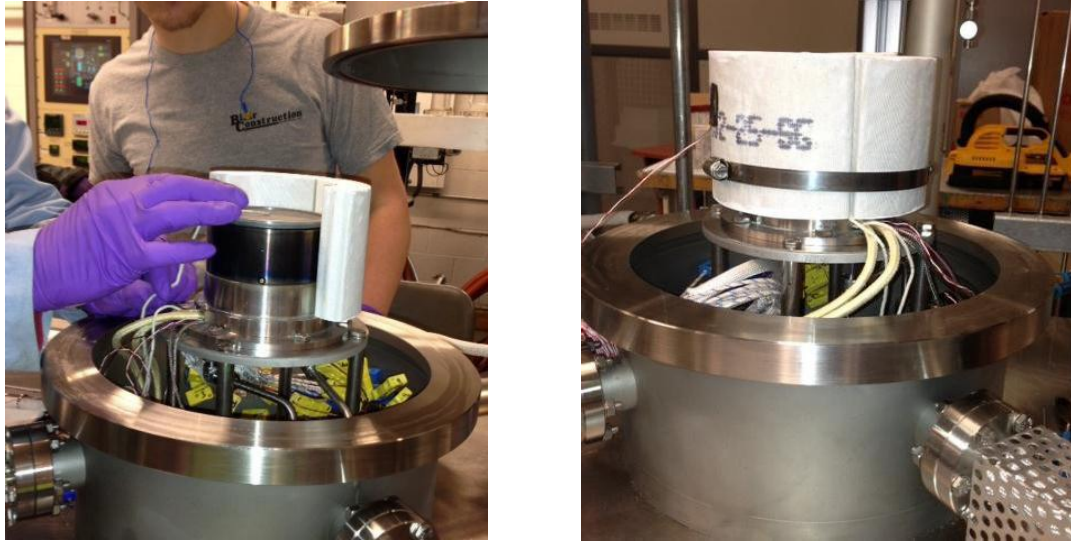
Figure 4.—Moulded Pipe Section (MPS) holder installed around tungsten heater in multilayer insulation (MLI) rig. Image on left shows MPS holder being installed around the heater. Image on right shows MPS holder in its testing configuration.
