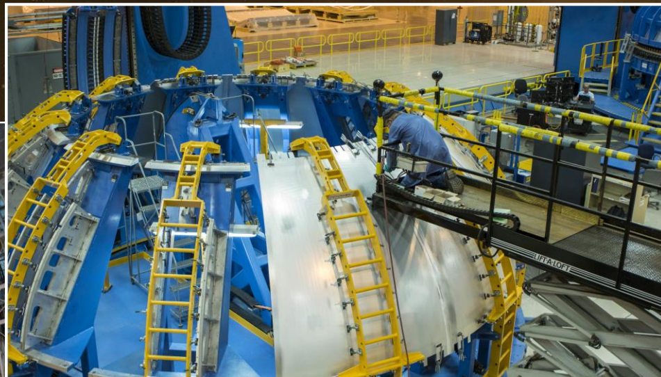
LH2 Dome Assembly at Michoud
