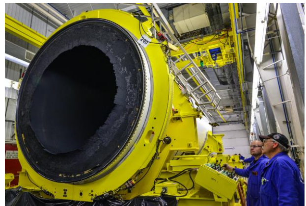
Fig. V: Orbital ATK workers detach center-forward segment of QM-1 motor test fired at the company's Provo, Utah facility.
