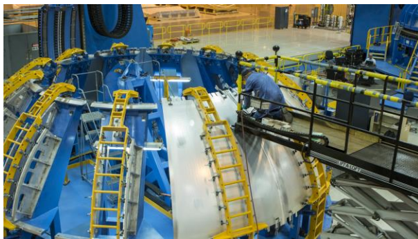
Figure VII: Vertical Assembly Center (VAC) (top) and LH 2 tank dome on Gore Weld Tool (bottom) at Michoud Assembly Facility.
