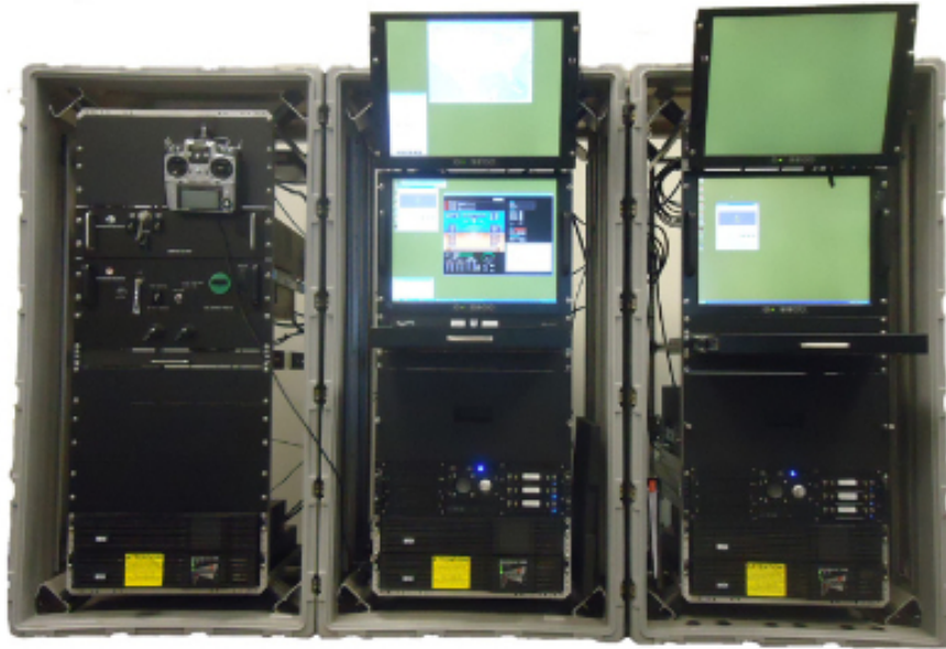
Figure 4.3: Ground simulation and testing system for the Viking 400 UAS
