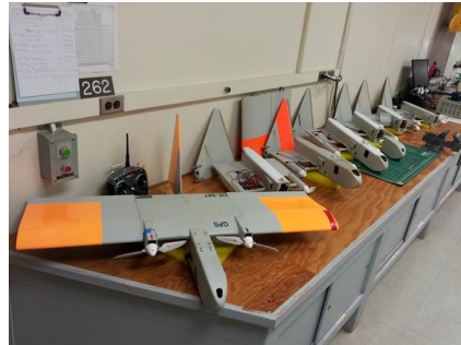
(c) Assembled DragonEye test vehicle next to array of spare parts in N-211 test laboratory
