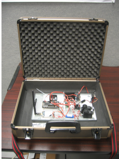
Figure 4.2: Ironbird ground test system for modified Dragon Eyes
