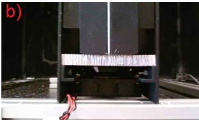
Figure 5. Forced-flow configuration. a) Front view of sample card placed on top of fans. b) Side view showing the fan bank at the bottom, the 1.5-cm-thick honeycomb flow straightener, and the sample card above.
