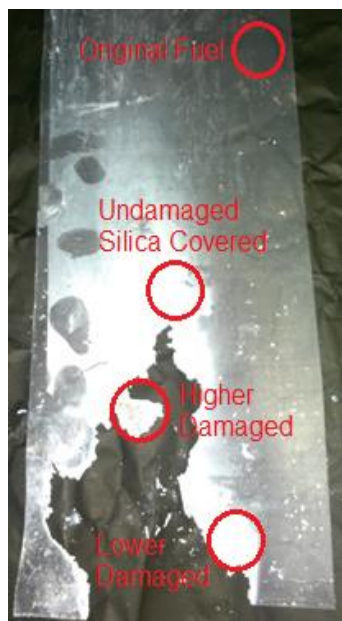
Figure 10. Sample of burned, originally 0.61-mm-thick silicone. Pieces at given distances away from the leading edge circled in red were cut out and analyzed using TGA.
