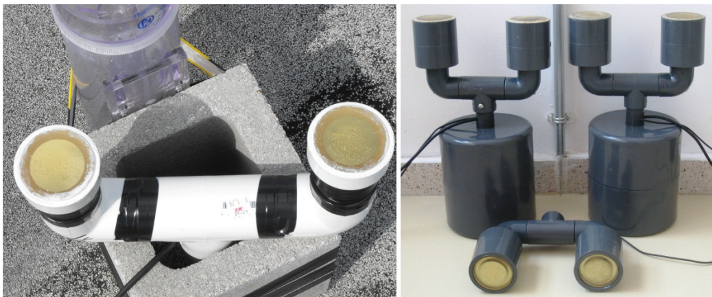
Fig. 4. (Color online) Dual head disdrometer design using largest available COTS piezoelectric disk, the muRata 7NB-41-1. Left: UCF prototype; Right: refined CUT version.
