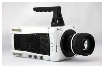
Figure 5: Phantom v411 wide-screen digital high speed camera to track angular deceleration versus time.
