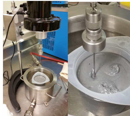
Figure 7. Setup of Viscometer, T-bar Spindle and propellant simulant test sample.
