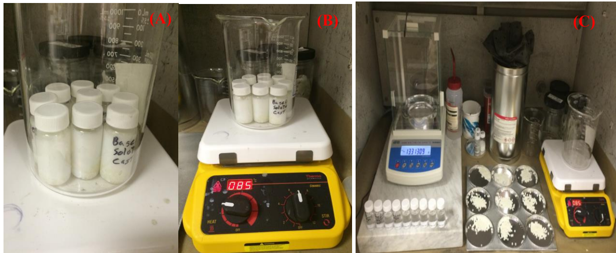
Figure 3. (A) The ABS acetone mixture placed in beaker before placement on the mechanical stirring heat plate. (B) Beaker placed on magnetic stirring heat plate for eight hours. (C) Overall experiment setup for ABS pellet material modifications infusion process.
