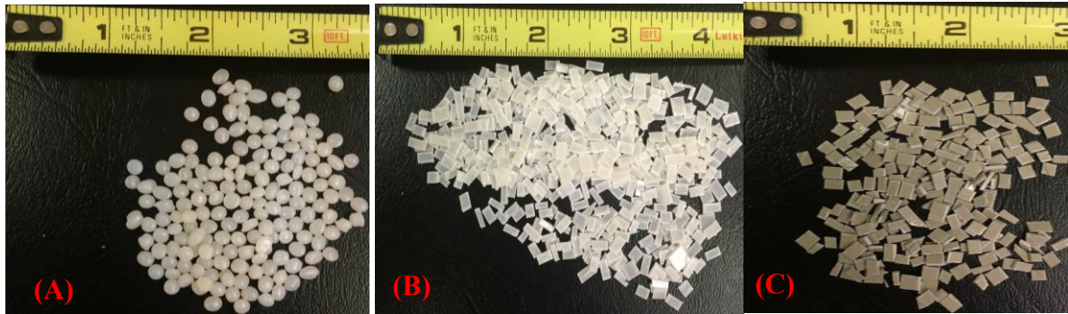
Figure 5. (A) ABS pellets before acetone addition. (B) Solution cast ABS wafer after being dissected into chips for insertion into the Filabot hopper. (C) Solution cast ABS and SiC infusion wafer after being dissected into chips for insertion into the Filabot hopper.
