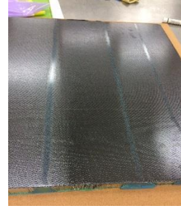
Figure 3. Cured 2' x 2' spliced demonstration sandwich panel.
