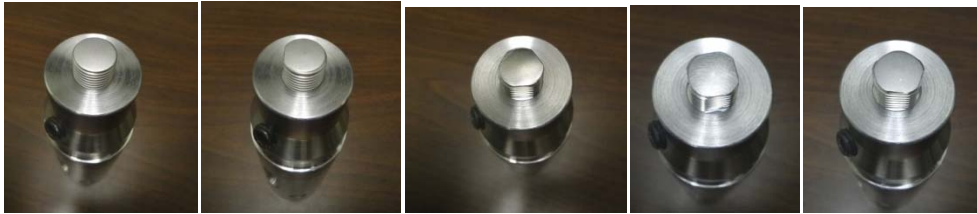
Figure 1. The sets of tool geometries evaluated in this study using a threaded pin with varying number of flats.
