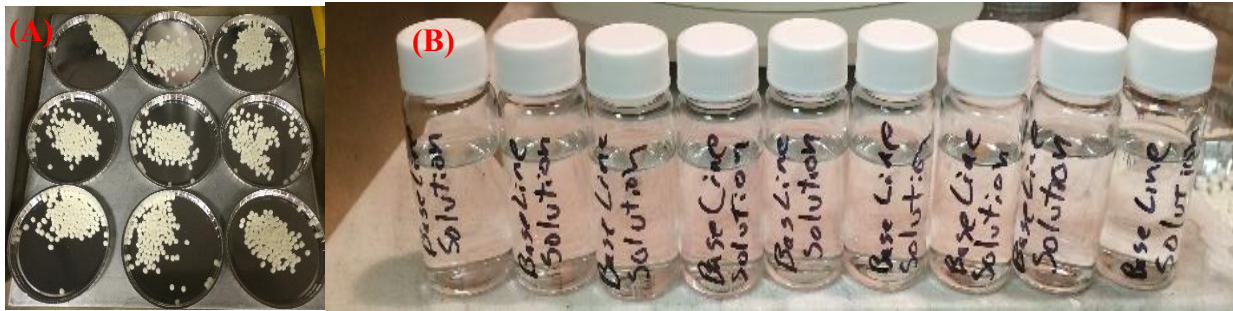
Figure 1. (A) 30 grams of ABS pellets separated into aluminum dishes before being added into the vial of Acetone (B) 90 grams of acetone in vials before mixing with ABS pellets.
