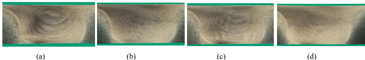
Figure 2. Transverse FSWs comparing with a threaded pin with no flats (a), 3 flats (b), 1 flat (c) and 5 flats (d).
