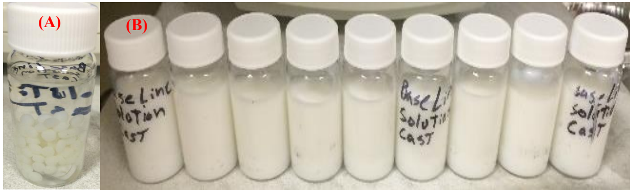
Figure 2. (A) 30 grams of ABS pellets before being fully dissolved into 90 grams of acetone. (B) ABS acetone mixture before being magnetically stirred dissolved in 90 grams of acetone.
