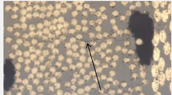
Microcracks formed in thin plies primarily due to presence of porosity
