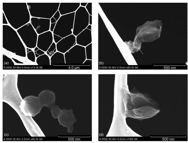
Figure 17.—High resolution SEM analysis of Kapton smoke particles at 640 °C on a lacey carbon TEM grid showing irregular surfaces and angular edges. (a) Typical coverage. (b) Approximately 700 nm long. (c) The coating on spherical particle chain appears to have primaries connected by liquid bridges that solidified and connected primary particles ranging from 100 to 350 nm. (d) 500 nm particle.
