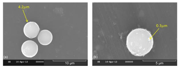
Figure 7.—SEM images of wire insulation smoke particles at 640 °C (Run 6). These large spheres range from 4.0 to 4.6 µm diameter. (a) Three spherical particles in proximity. (b) Note the smaller particles adhered to the large particle.
