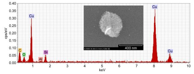
Figure 20.—EDS spectrum of a 400 nm Kapton smoke particle (inset) at 640 °C on a carbon film TEM grid showing Cu, Si, and Al. The Al is most likely a system peak, Cu can be attributed to the copper TEM grid and Si is potentially from the mica liner in the WSTF smoke generator.
