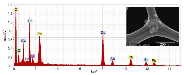
Figure 3.—EDS spectrum of a circuit board smoke particle at 540 °C with TEM grid image (inset) (Run 31).
