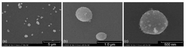
Figure 8.—High resolution SEM images of Teflon smoke particles at 540 °C collected onto a carbon film TEM grid. (a) 250 nm to 1.5 μm diam. range. (b) 500 nm and 700 nm diam. (c) 700 nm diam.
