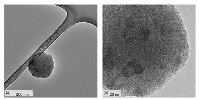
Figure 12.—High resolution TEM images of a Teflon smoke particle at 640 °C (test 15) adhered to a lacey carbon TEM grid. (a) Compact agglomerate, approximately 250 nm diam. contains smaller particles bound together by amorphous material. (b) Particle detail.
