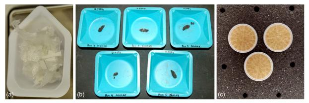
Figure 28.—Nomex fuel tests. (a) Nomex snips before heating (0.5 g fuel sample). (b) After heating, the Nomex snips became one or two compact pieces of char/ash, as shown in the remains of five different tests. (c) TEOM filters after mass concentration measurements of Nomex smoke particles show the characteristic yellowish color of brown carbon.
