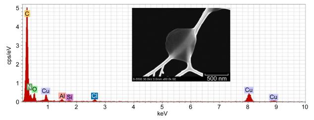
Figure 25.—EDS spectrum of a non-spherical 700 nm Nomex smoke particle with a rounded irregular shape (inset) containing C, O, N, Al, Si, and Cl. The Al may be a system peak, Cu can be attributed to the copper TEM grid and Si is potentially from the mica liner in the WSTF smoke generator.
