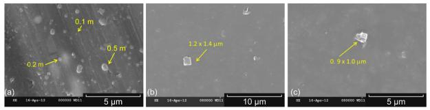
Figure 6.—SEM images of wire insulation smoke particles at 640 °C (Run 6). (a) Smaller particle populations are mostly spherical. (b) and (c) Particles with square crystalline morphology.
