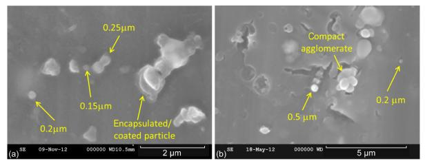
Figure 1.—SEM images of circuit board smoke particles. (a) At 640 °C (Run 33). (b) At 340 °C (Run 27).
