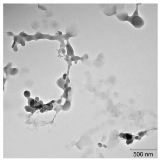
Figure 15.—Teflon smoke particles collected with the SAME thermal precipitator on the ISS, showing vastly different morphology compared to WSTF samples (TEM, Philips Model CM20).
