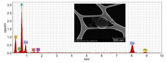
Figure 10.—High resolution SEM image of Teflon smoke particle (inset) at 540 °C collected on a lacey carbon TEM grid and corresponding EDS spectrum with a prominent F peak.
