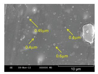
Figure 22.—SEM image showing spherical Nomex smoke particles in the 300 to 600 nm range and a large irregular particle (on the right), possibly char. Light areas indicate charging by the electron beam, however, the spherical particles are stable and did not volatilize under the beam.
