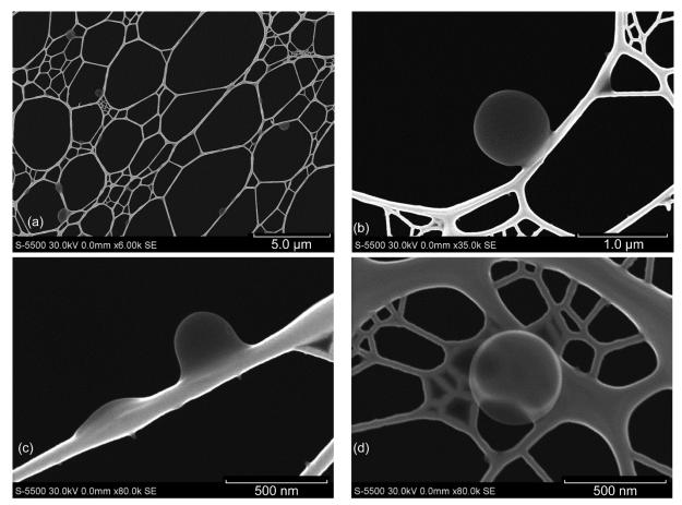
Figure 26.—High resolution SEM images of Nomex smoke particles that appear on the TEM grid as liquid droplets of varying solidity, some with perfectly spherical tar ball morphology. Diameters of single particles range from 300 to 800 nm. (a) Large scale image showing coverage (b) 800 nm. (c) 300 nm. (d) 450 nm.
