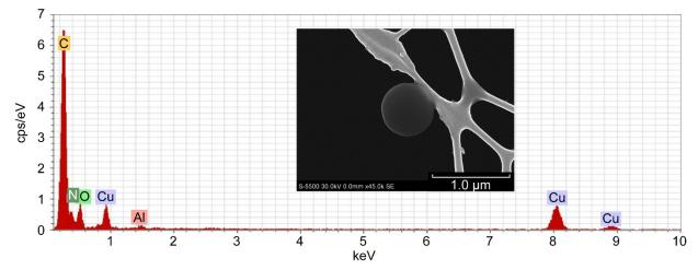
Figure 27.—EDS spectrum of a tar ball-like 600 nm Nomex smoke particle (inset) with peaks of C, O, N, Al, Si, and Cl.
