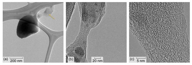
Figure 11.—High resolution TEM images of a Teflon smoke particle at 640 °C (test 15) adhered to a lacey carbon TEM grid. (a) The irregular rounded particle with an extended tail is approximately 400 nm in diameter. (b) Particle tail detail which contains smaller particles. (c) Amorphous interior structure of the tail.
