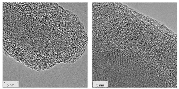
Figure 14.—High resolution TEM images of a Teflon smoke particle at 640 °C (test 15) showing a crystalline interior with an amorphous coating.
