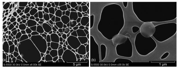
Figure 9.—High resolution SEM images of Teflon smoke particles at 540 °C collected onto a lacey carbon TEM grid. (a) Representative particles. (b) 700 nm and approximately 400 nm diam.
