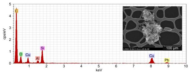
Figure 5.—EDS spectrum of circuit board smoke particle (inset) at 540 °C (Run 31) and TEM image. The jagged crustal particle is much larger than the typical rounded particles and EDS shows a significant Si peak as well as Cu and AI, all typical constituents of electronics (circuit board and components).
