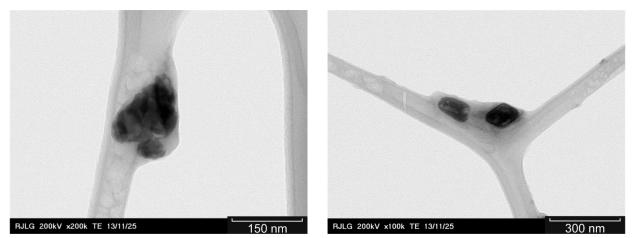
Figure 4.—High resolution STEM image details on inclusions within circuit board smoke particles at 540 °C (Run 31).
