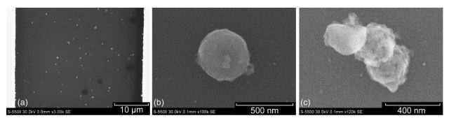
Figure 19.—High resolution SEM images of Kapton smoke particles at 640 °C. (a) Typical coverage. (b) 450 nm spherical particle with multiple smaller particles adhered to it. (c) Chain of three particles all close to 350 nm diam.
