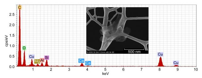
Figure 24.—Spectrum of an irregular Nomex smoke particle with distinct angular inclusions (inset), containing O as well as the elements, Si, Ca, Al, and Mg. The Al may be a system peak and Cu can be attributed to the copper TEM grid.
