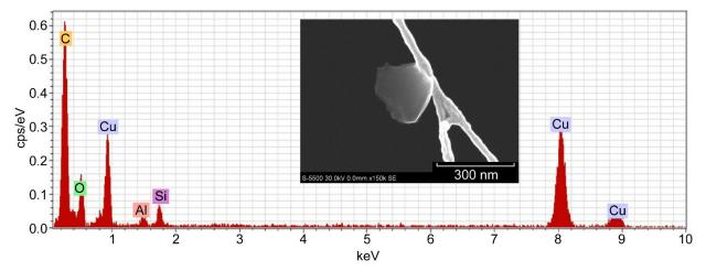
Figure 18.—Angular Kapton smoke particle (inset), approximately 270 nm at 640 °C with its EDS spectrum showing O, Si, and Al. The Al is most likely a system peak, Cu can be attributed to the copper TEM grid, and Si is potentially from the mica liner in the WSTF smoke generator.
