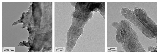
Figure 13.—High resolution TEM images of a Teflon smoke particle at 640 °C (test 15).
