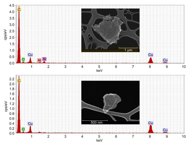
Figure 23.—SEM images and corresponding spectra from Nomex smoke of what appear to be char particles owing to the high C peaks. Cu in both spectra are attributed to the copper TEM grid in the upper spectrum.
