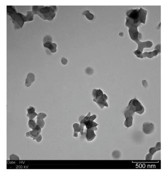
Figure 21.—Aged Kapton smoke particles collected with the SAME thermal precipitator on the ISS showing similar morphology to WSTF samples (TEM, Philips Model CM20).
