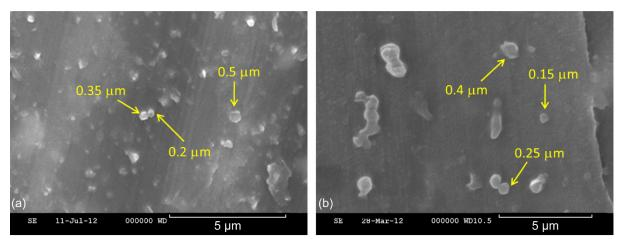
Figure 16.—SEM images of Kapton smoke particles on the AI SEM stub. (a) At 540 °C are compact and either spherical or angular. (b) At 640 °C exhibit chain-like agglomerate structures, some doublets and longer chains are coated.
