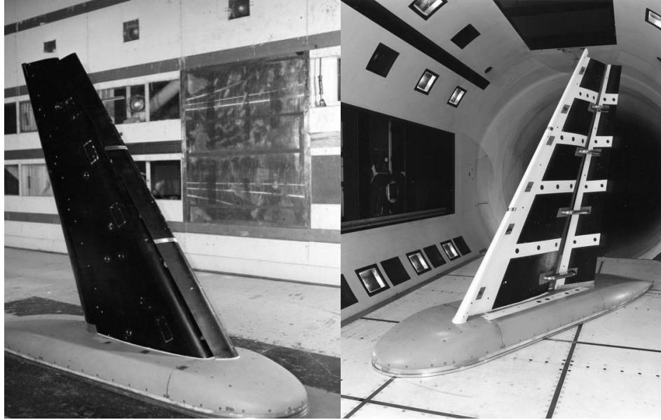
Figure-2.2.1: NASA Trap Wing Geometry in the wind tunnel (Image reference: AIAA HLPW-1)
