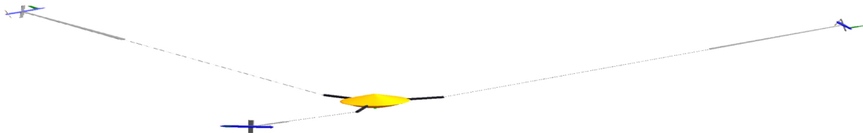
Figure 2.1: Complete Centrifugally Stiffened Rotor (CSR) system.
