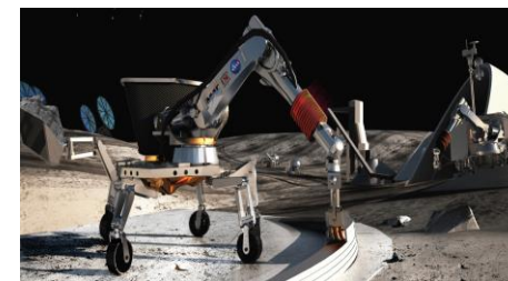
Concept of ATHLETE-based autonomous additive construction system on extraterrestrial surface
