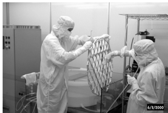
Fig. 4-20. Rinse water from array frame is captured in beaker for particle counting analysis.
