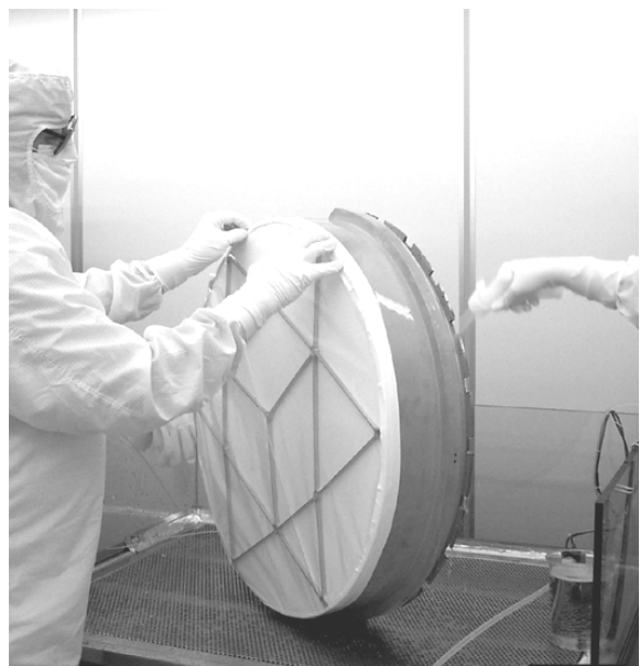
Fig. 4-11. Unpainted portion of canister cover is rinsed with UPW. Painted portion is covered with film Teflon taped at rim.
