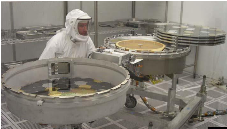
Fig. 1-3. Fully open canister revealing deployed arrays and concentrator (in center).
