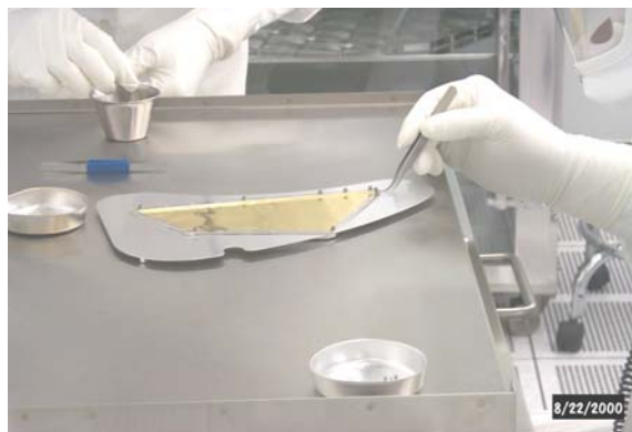
Fig. 5-6. During assembly, fasteners were handled with tweezers, not gloved fingers.
