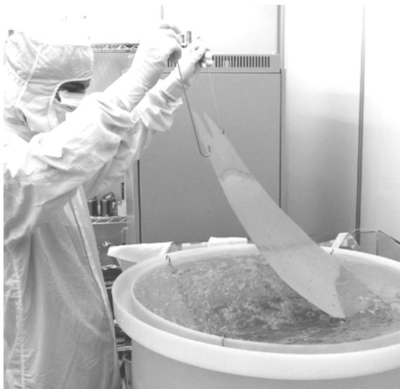
Fig. 4-22. Gap shield being lowered into UPW cascade bath.
