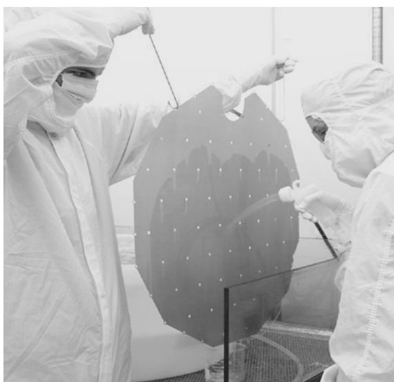
Fig. 4-24. Rinse water being captured for particle count analysis and measurement of organic content.
