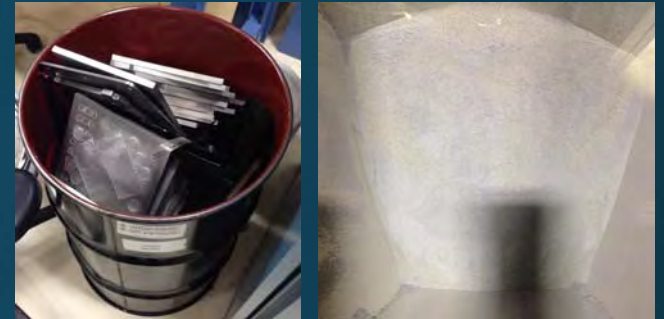
Spent build plates and oversized powder
