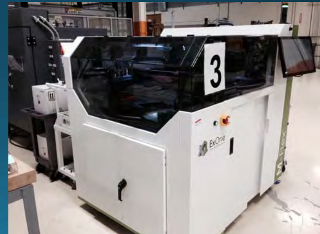
ExOne M-Flex Binder-Jet at ORNL MDF
