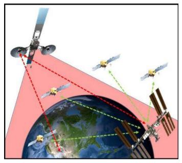
The Next Generation Broadcast Service (NGBS), formally known as the TDRSS Augmentation Service for Satellites (TASS), will demonstrate a forward beacon that can be utilized for the sending and receiving of critical UIS communications, individual mission data, and radiometrics or optimetrics for onboard navigation.
