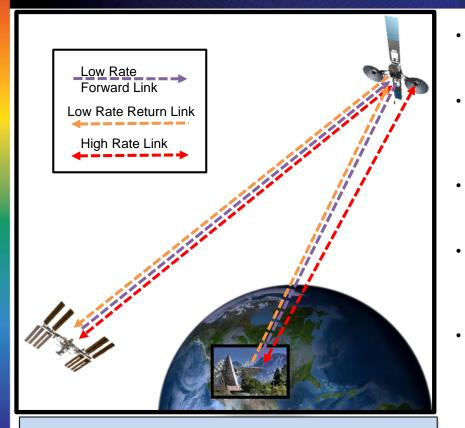
SMN Provides Continuously Available Forward and Return Links and Enables Users to Schedule High Data Rate Forward and Return Links through User Initiated Services (UIS), a revolution in mission execution.
