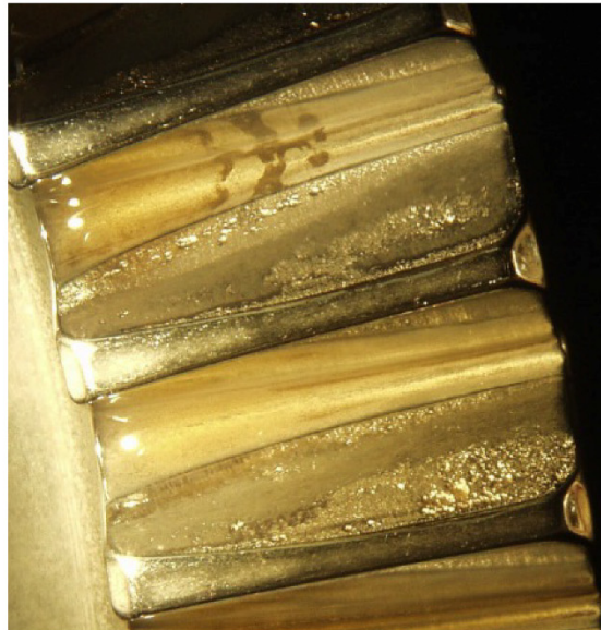
Figure 12.—Typical contact fatigue failures of ISF test gear sets. (a) Pinion failure, contact fatigue, macropitting, spall. (b) Pinion failure, contact fatigue, macropitting, progressive. (c) Face gear failure, contact fatigue, macropitting, progressive.
