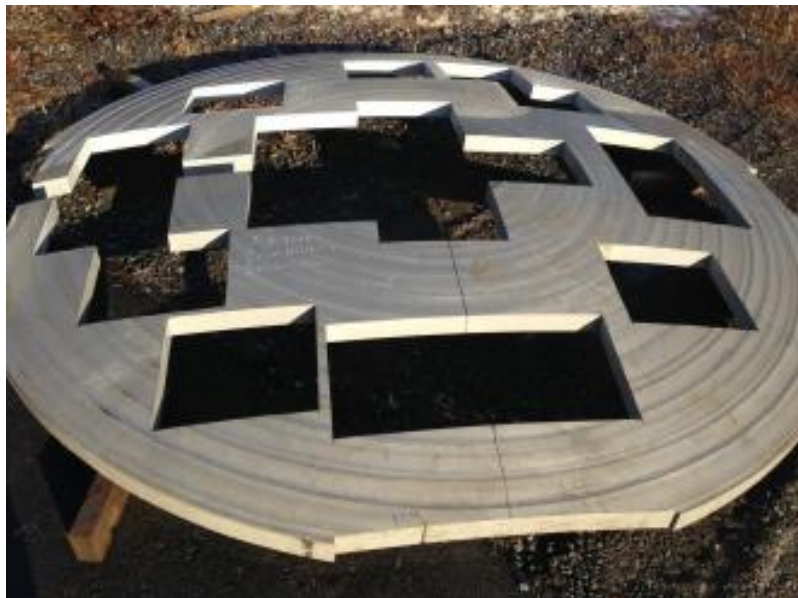
Figure 7.10-2. Aft Bulkhead following Extraction of Coupon Blanks for Test and Analysis
