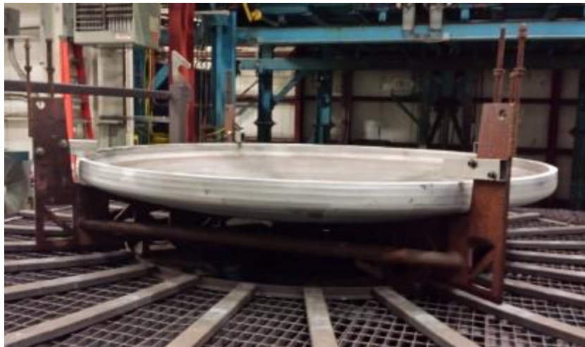
Figure 7.8-1. Aft bulkhead following heat treatment.
