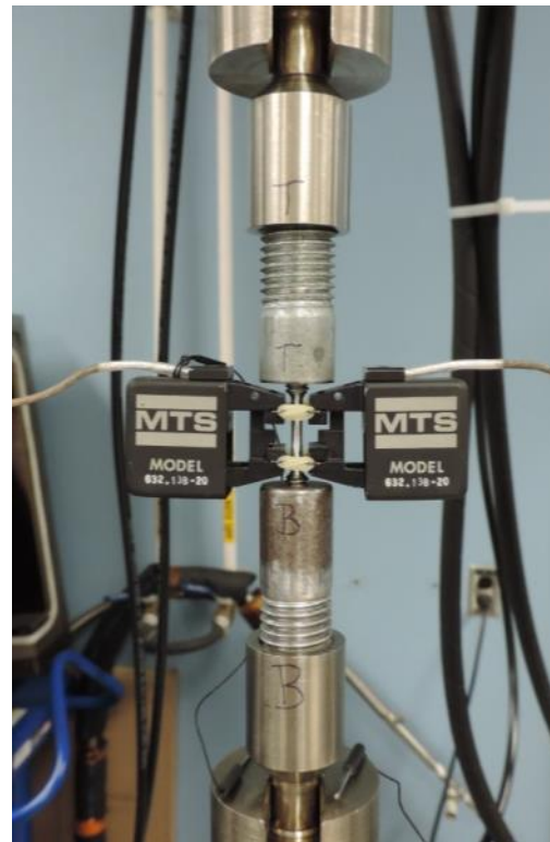
Figure 8.3-4. Tensile Test Load Stand, Specimen, and Instrumentation
