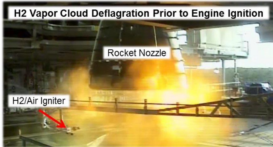
Figure 34: RS-25 Engine External Ignition at the SSC A-1 Test Stand
