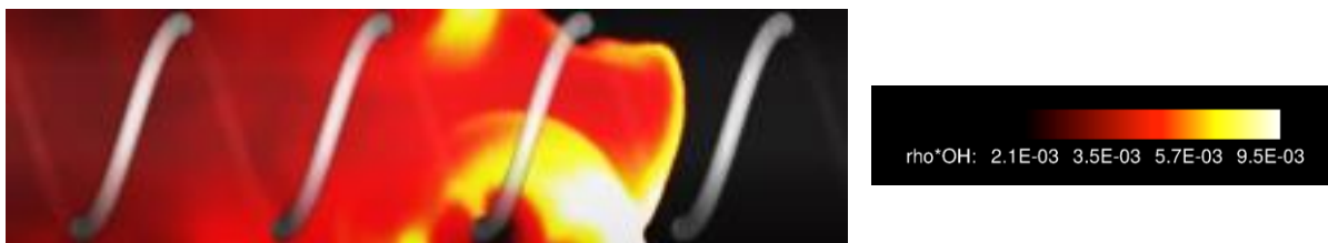
Figure 32: Localized Explosion Events Predicted During the Onset of Detonation (Visualized by Center-Plane Cut of \rho \cdot Y_{OH} )
