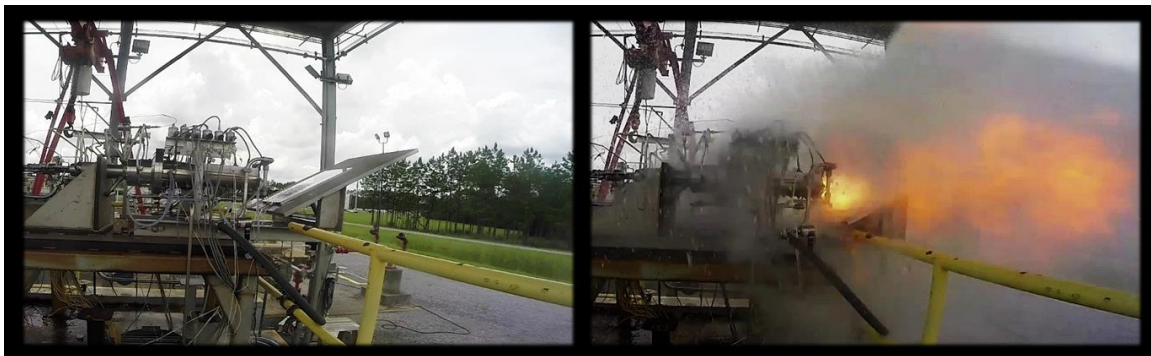
Figure 45: Detonation Event during Altitude Diffuser Testing - (Left) Prior to Start and (Right) Detonation Wave Exiting Diffuser
