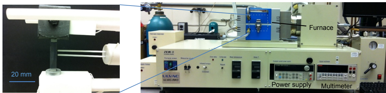
Figure 1.—ULVAC ZEM3 unit used for low/intermediate-temperature, isothermal characterization of SiC f /SiC specimens. On the left is a close-up showing specimen and four-point probe configuration (note: entire specimen housed within furnace).
