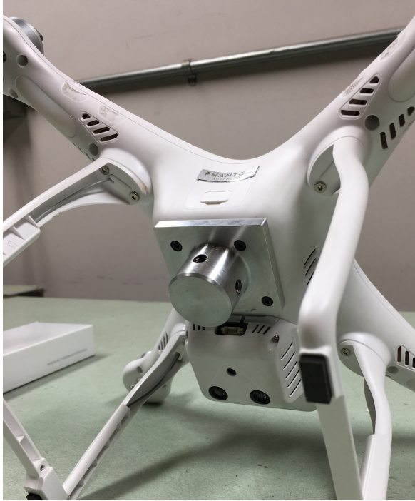
Figure 11. Model mounting plate for DJI Phantom 3.
