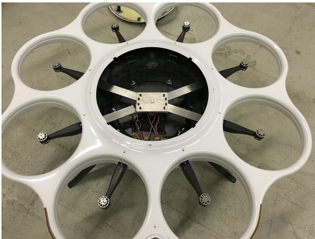
Figure 12. Drone America x8 internal mounting hardware.
