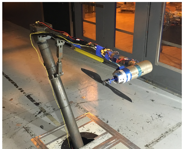
Figure 7. Isolated rotor – SUI Endurance.
