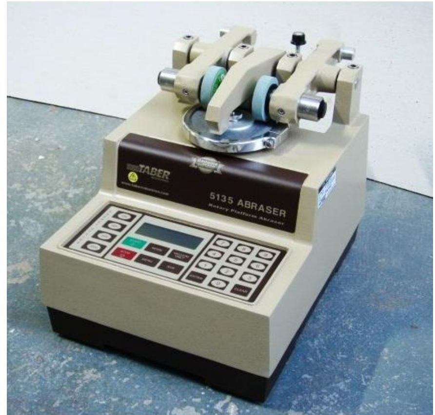
ASTM D 3884-01 test device
