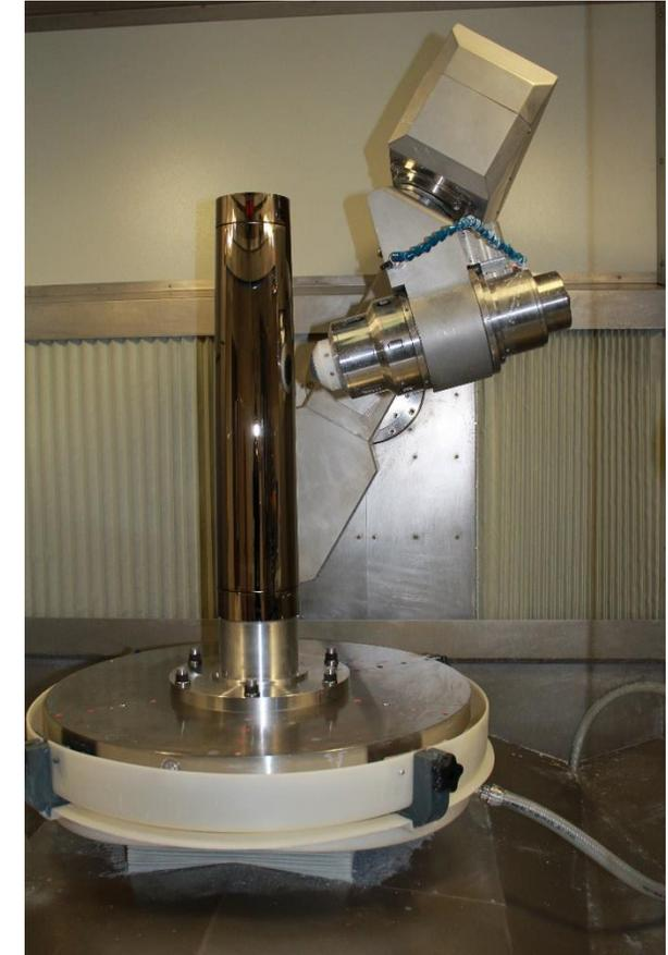
ART-XC mandrel installed on the Zeeko machine for figuring experiments
