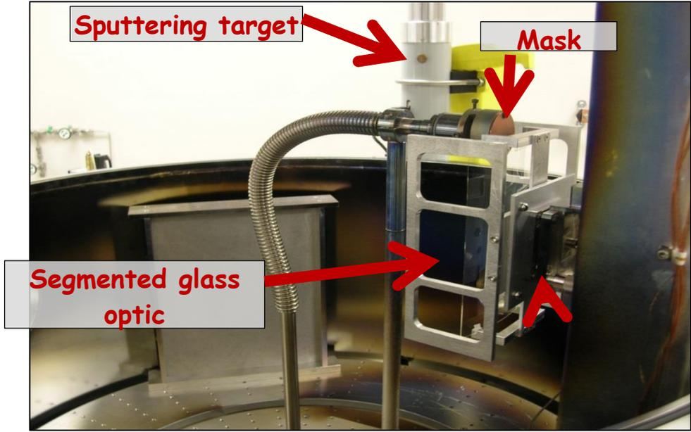
**Recent X-ray test results:** Angular resolution is improved from 17 to 20 arc secs to  $\sim 5$  arc secs HPD.
