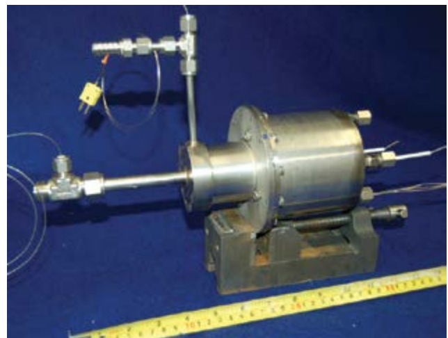
HMC source contaminant control catalytic oxidizer.
