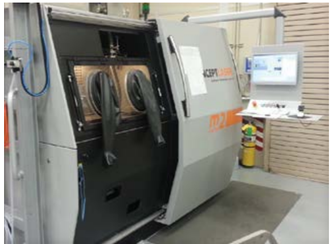
Figure 1: SLM machine with glovebox required for Ti64.
