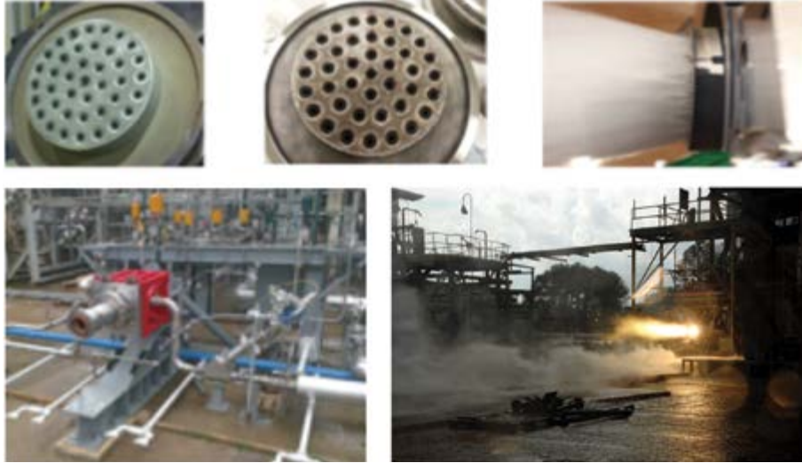
Figure 2: Water flow and hot-fire testing of two LOX/H 2 SLM injectors.
