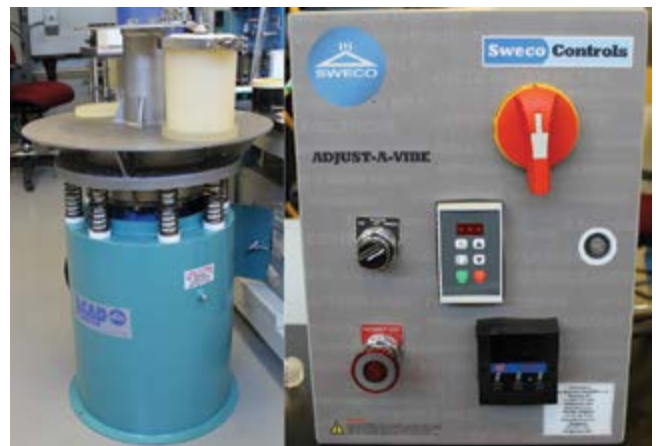
Vibratory mill and control system.
