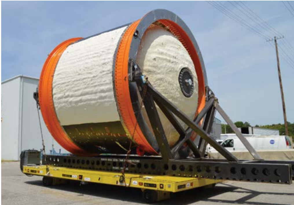
CCTD in-transit on TPS transporter—foam application is complete on domes and main barrel section.
