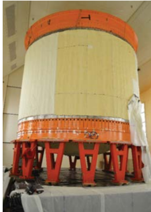
5.5-m-diameter CCTD in vertical orientation following completion of foam application.
