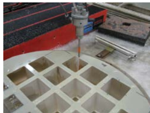
MOR specimens in abrasive waterjet cutting.
