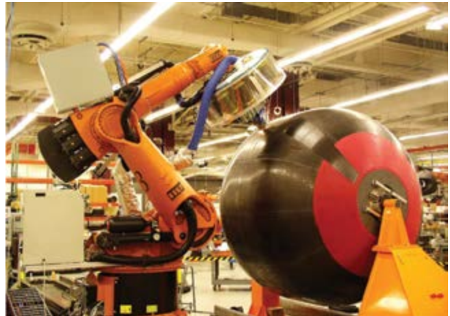
Figure 1: 8-ft- (2.4-m-) diameter, all composite tank at Boeing.
