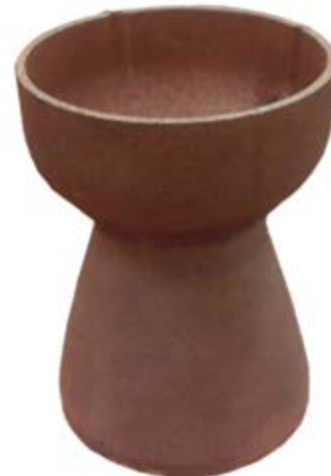
Small chamber process demonstration article printed by MSFC ER42 from copper alloy C18150.
