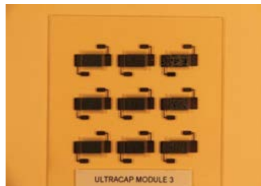
Ultracapacitor single cells printed using 3D aerosol jet printing—the first board printed using multiple single cells to test scalability.
