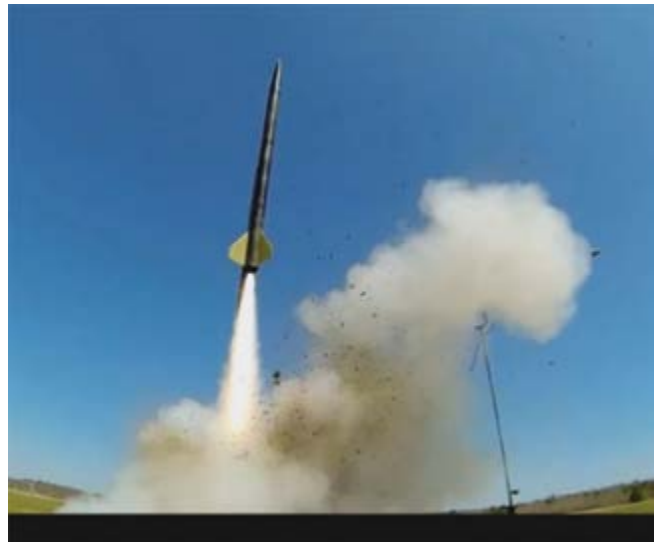
Figure 1: Local test flight of the Avionics and RCS on the NL1D ('Wildman' amateur hobby rocket kit w/M3400 motor).
