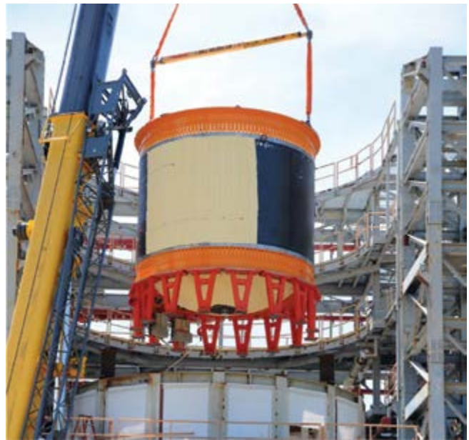
Figure 1: 18-ft- (5.5-m-) diameter, all composite tank at MSFC.
