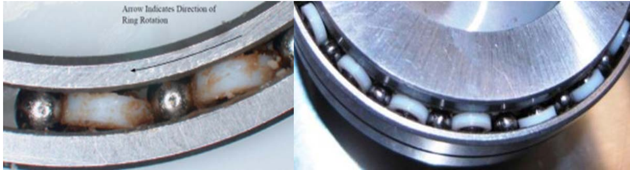
Figure 5. Comparison of Test Station#2 bearing with a similar bearing in relatively good condition with equal direction reversals after 6X times the number of revolutions.
