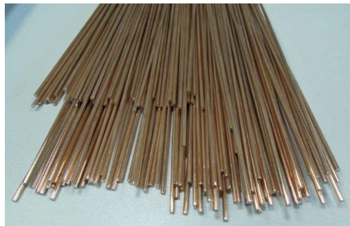
Figure 1. Cu-Al-Ni single crystal \varnothing 2.2-mm wires made with special Nimesis process
