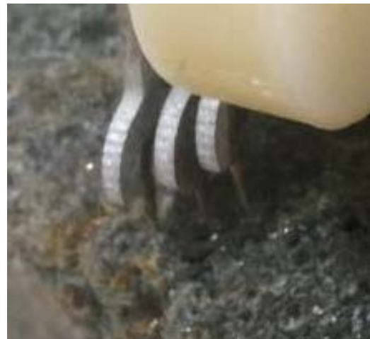
This photo shows a hook that has shifted in its mounting epoxy due to a high transverse load.
