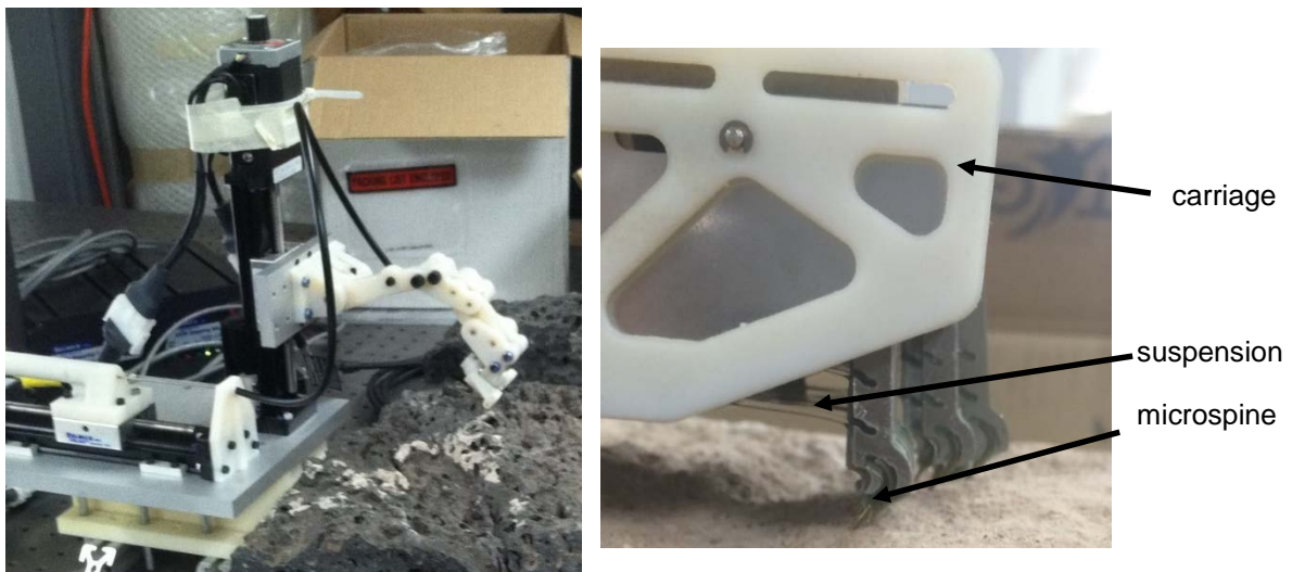
Figure 9. Testing on the microspine gripper in a test fixture. Top: The entire test fixture, with independent x- and z- stages to test gripping force in each direction (the rock is scoria). Bottom: Close-up view of microspines during testing (the rock is rhyolite).
