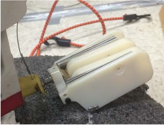
The original test gripper experienced interference with the rock sample, necessitating a redesign that provided adequate clearance.
