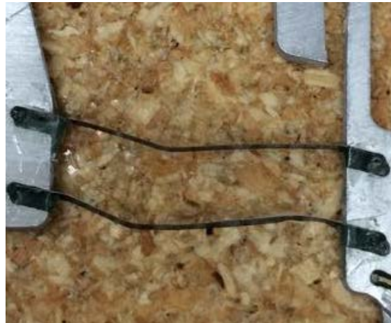
If an x-direction compression load is exerted on the z-direction flexures, this crimping failure can result, indicating the need to protect the flexures from compressive loads.
