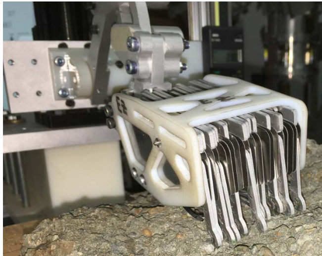
Test run incorporating divider sheets to reduce tangling.
