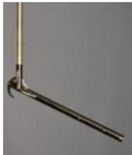
Articulated sensor developed for profilometry of domes
