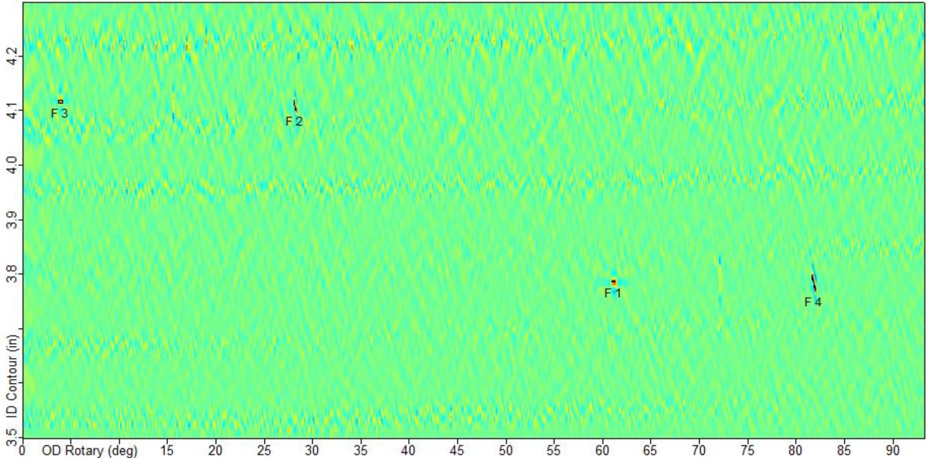
Linear FIR filter applied - optimized for Circumferential flaws
