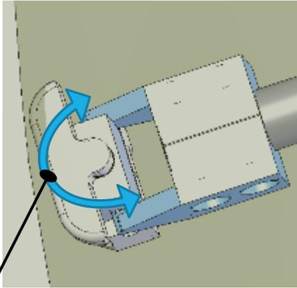
Surface-riding assembly pivots to maintain contact on domes
