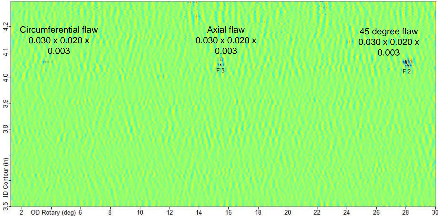
Rotary FIR filter applied - optimized for axial flaws
