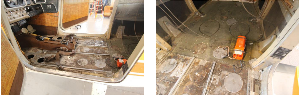
Figure 6 - Test 1 original airplane ELT beacon installation as viewed from the pilot door (left) and pilot seat looking aft (right)
