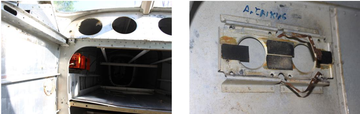
Figure 25 - Test 3 original airplane ELT location (left) and aircraft attachment plate (right)
