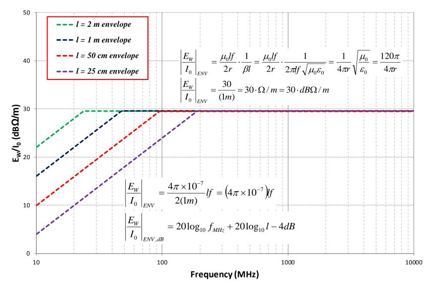
**Ground Plane Attenuation Horizontal Polarization Only)**
