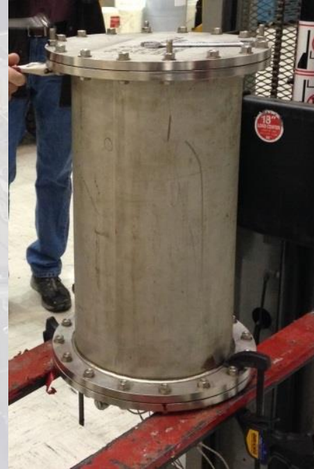
Batch Carbon Formation Reactor – closed (left) and during steel bead packing (right)
