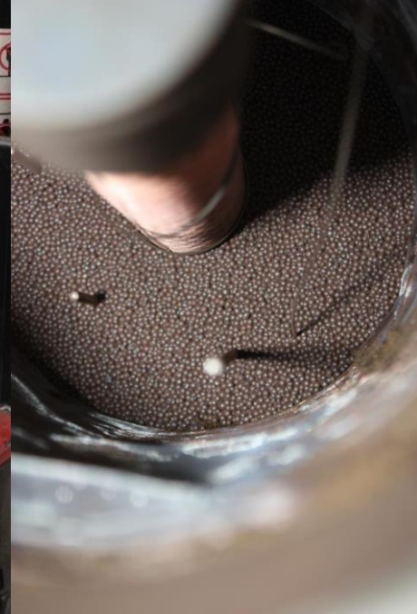
Batch Carbon Formation Reactor – closed (left) and during steel bead packing (right)
