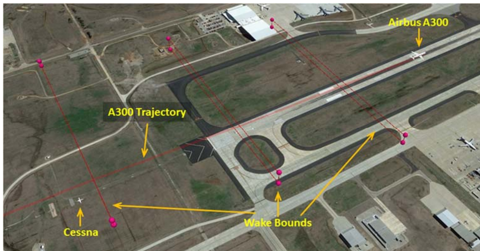
Figure 4.6. Cessna encountering the wake bounds predicted by the APA simulation.
