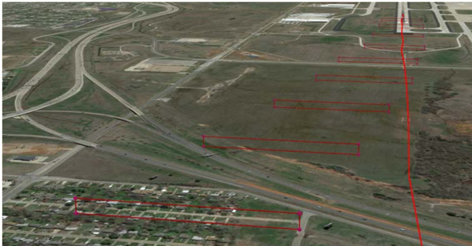
Figure 4.5. Transport of A300 wake by crosswinds predicted by the APA simulation.
