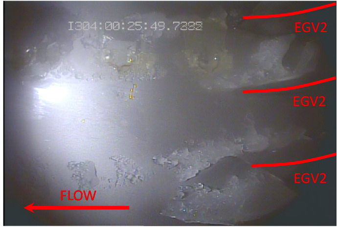
Figure 12.—Example of accretion for FLT850 nonrollback.
